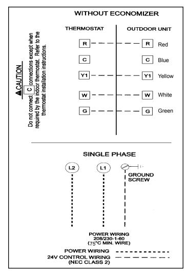
**Figure 6. Typical Wiring Connections**
