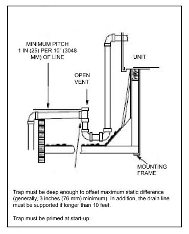
Figure 3. Typical Condensate Drain Connection
