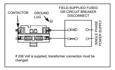
Figure 5. 208/230 Line Voltage Wiring
