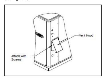
Figure 2. Installing the Vent Cover
