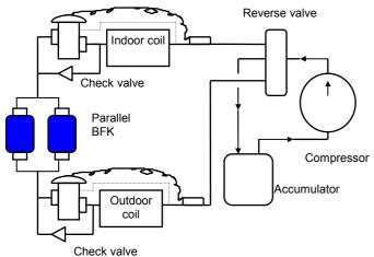
4. Heat pumps with Bi-flow expansion valve
