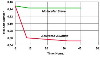
There are different types of Activated Alumina. The application of these adsorbents are dependent on the manufacturing process, binding material and style such as block or compacted beads. Alco BFK incorporated a type of Activated Alumina with very high organic acid adsorption capacity.
