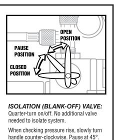
Valve is completely closed at 90°.
