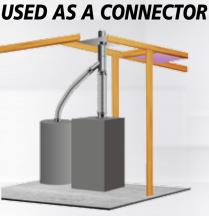
Make a direct connection from one or both appliances to a common B-Vent.
