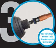
With power tool at MAX speed push bit into the refrigerant line. Keep bit centered & push until the stopper bottoms out, then remove bit from line.
