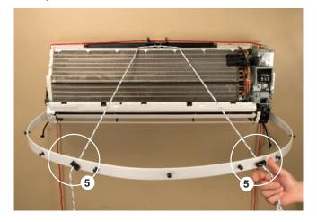
**6.** Attach the single-use Funnel Bag to the frame by rolling it over the C-Band from the inside. Secure the mounting holes in the bag to the mounting studs along the C-Band. **V**
