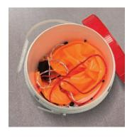
U.S. Patent No. 6,863,116 Under license from Crossford International LLC After cleaning, unhook C-Band with the single-use Funnel Bag attached. Roll entire assembly into Drain Pail. Remove Drain Pail outdoors and separate the bag from the frame.
